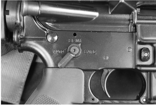
Figure 4.39 A close-up of the right side of an AR-15 lower receiver. Note the three positions of the selector switch: SAFE, SEMI, AUTO. The hole above the SEMI position is for the auto sear pin. Although no sear is installed in this gun and the pin hole is empty, the mere presence of this hole would define this receiver as a machine gun. (Image from author's collection.)
